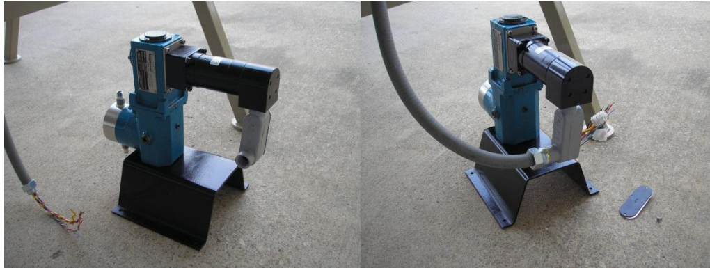
Figure 2.12: Chemical Pump Conduit Fitting
